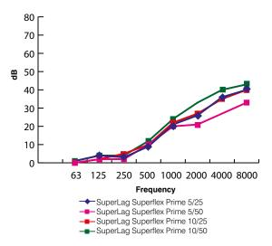
The acoustic performance of CMS Danskin Acoustics SuperLag Superflex Prime can further enhanced by applying on top of a layer of glass fibre slab up to 300mm thick where very high performance levels are required.
