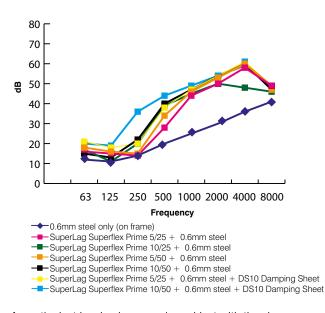
Acoustic duct lagging is a complex subject with the size, shape, thickness and configuration of the ductwork all having a significant effect on the system performance. The data shown above is based on flat panel tests used for SuperLag Superflex Prime products.
